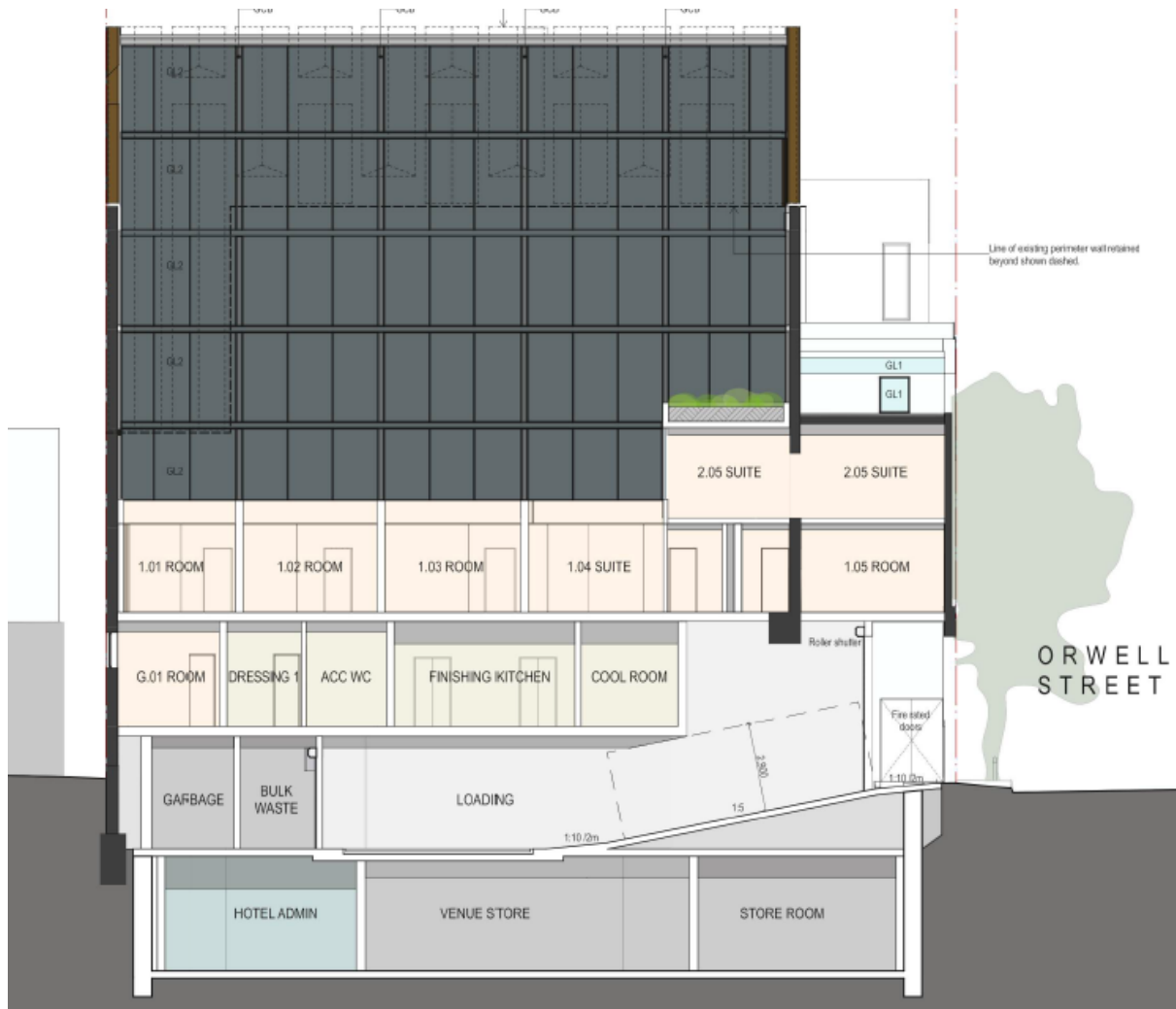
Figure 34: Section through the fly tower
